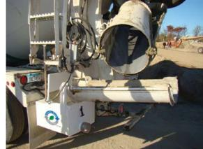
Recover and recycle wash water back into the truck
